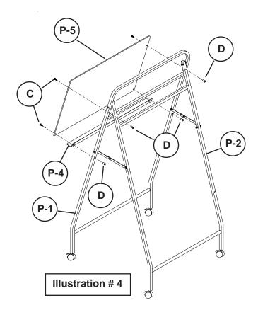
6. Assemble Marker Board (P-6) by inserting 5/8" Socket Screw (C) through the Marker Board (P-6), and Board Tray (P-4). Insert board and tray through the Leg (P-2). Use the Screw Post (D) from the back of the leg and tighten with Allen Wrenches (H). See illustrations # 5.
