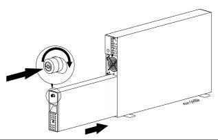
A Rotate the BATTERY ON/OFF switch in counter clockwise direction to turn on the battery pack.
