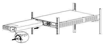
**6** Rotate the BATTERY ON/OFF switch in counter clockwise direction to turn on the battery pack.
