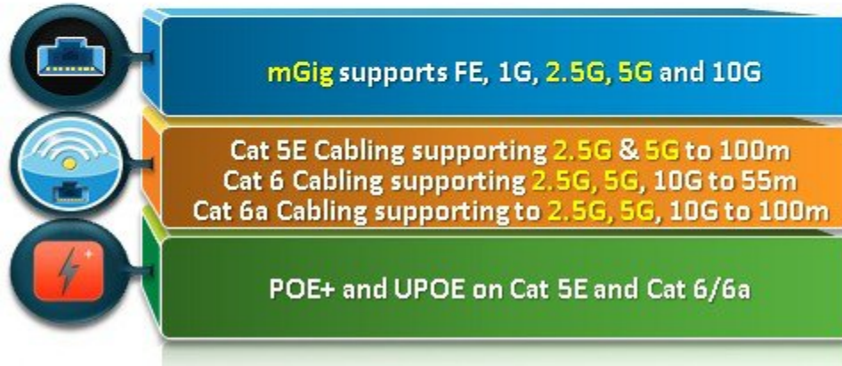
Figure 53: Cisco Multigigabit distance limitations
