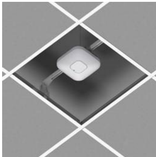
Figure 25: Oberon Model 1045- Above ceiling hanger kit - this includes a hanger bar and wire, and a light pipe that can be pressed through the ceiling tile so you can see the status LED from below, without lifting ceiling tile
