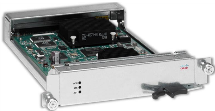
Figure 8. NCS5500/5700 modular platform system controller
