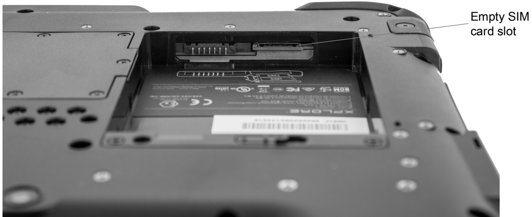
Figure 2 SIM Card Slot with Holder
