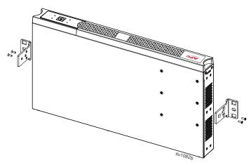
Note: Whenever possible, attach two screws into wall studs. If stud mounting is not possible, use an expandable wall anchor. Hardware is not included; 25" x 2" lag bolts are recommended. Mount the UPS in either of the displayed positions.
