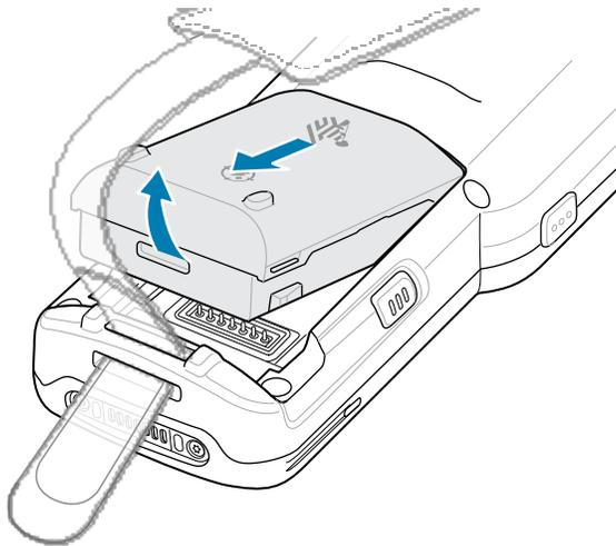
4. To install the battery, align the battery into the battery compartment.
