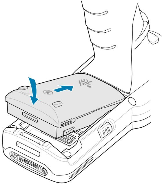
3. Slide the front of the battery into the battery compartment.
