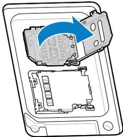
5. Place the SIM card into the cardholder with the contacts facing down.
