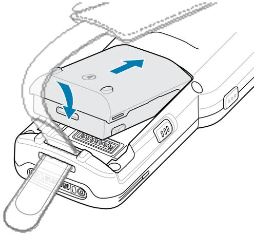
5. Slide the front of the battery into the battery compartment.
