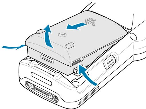
2. Using a coin or finger, remove the access cover.
