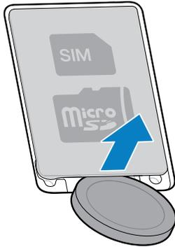
3. Slide the microSD card holder to the Open position.
