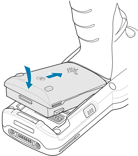
5. Slide the front of the battery into the battery compartment.
