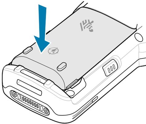
The device automatically resumes after battery removal and installation (in a Hot Swap change). The only time the Power key needs to be pressed is if the device has been powered off or left for a prolonged duration without a battery pack.
