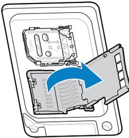
5. Insert the microSD card into the contact area with the contacts facing down.
