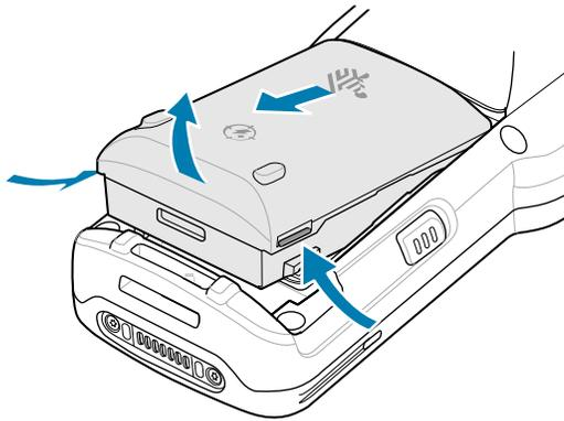
4. To install the battery, align the battery into the battery compartment.
