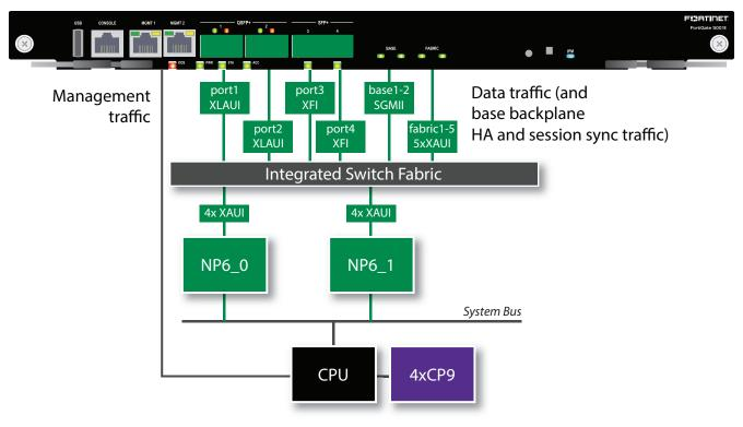
You can use the following get command to display the FortiGate-5001E NP6 configuration. The command output shows both NP6s connected to each interface with cross-chip offloading supported for all interfaces connected to the NP6 processors. You can also use the diagnose npu np6 port-list command to display this information.
