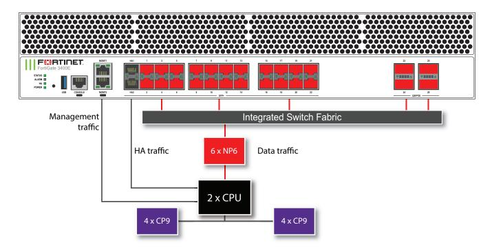
The MGMT interfaces are not connected to the NP6 processors. Management traffic passes to the CPU over a dedicated management path that is separate from the data path. You can also dedicate separate CPU resources for management traffic to further isolate management processing from data processing (see Improving GUI and CLI responsiveness (dedicated management CPU) on page 23).
