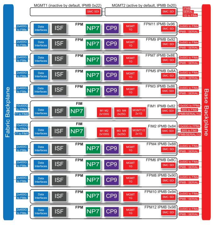
By default, MGMT2 is the active SMM and MGMT1 is inactive or passive. The active SMM always has the Intelligent Platform Management Bus (IPMB) address 0x20 and the passive SMM always has the IPMB address 0x22. Active and passive refers to the SMM that is controlling the chassis. The MGMT interfaces and console ports on both SMMs are always available.
