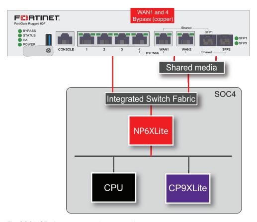
The SOC4 ISF allows you to use the command <code>config system virtual-switch</code> to create a virtual hardware switch that can include any front panel interface connected to the SOC4.
