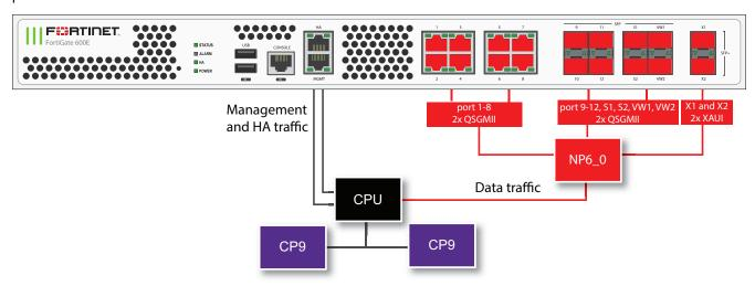
The FortiGate 600E and 601E each include one NP6 processor. All supported traffic passing between any two data interfaces can be offloaded by the NP6 processor. Data traffic to be processed by the CPU takes a dedicated data path through the NP6 processor to the CPU.
