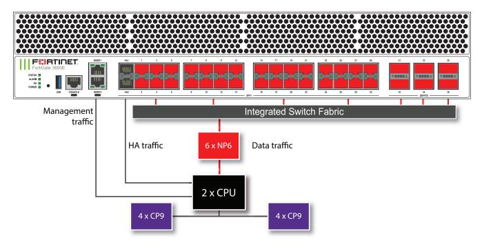
The MGMT interfaces are not connected to the NP6 processors. Management traffic passes to the CPU over a dedicated management path that is separate from the data path. You can also dedicate separate CPU resources for management traffic to further isolate management processing from data processing (see Improving GUI and CLI responsiveness (dedicated management CPU) on page 23).
