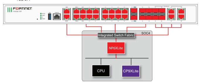
The SOC4 ISF also allows you to use the command <code>config system virtual-switch</code> to create a virtual hardware switch that can include any front panel interface connected to the SOC4.
