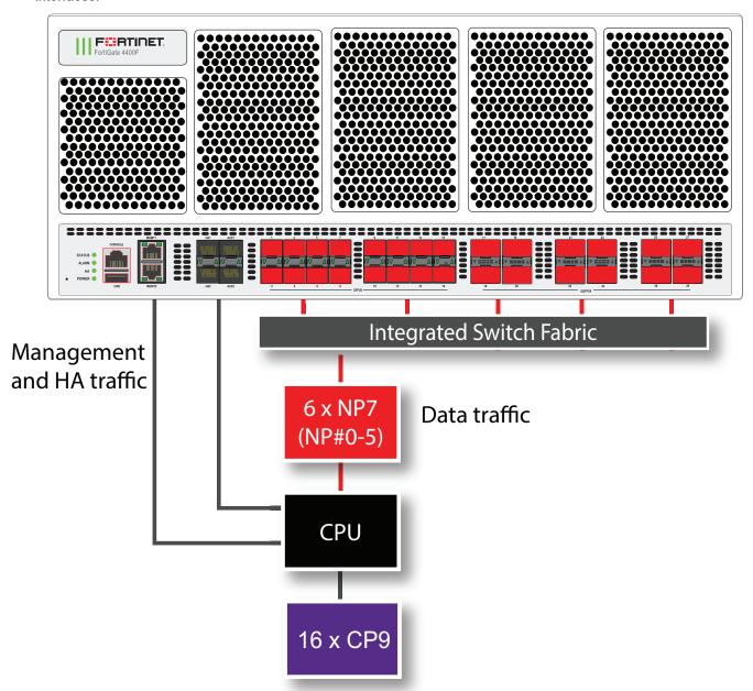
The MGMT interfaces are not connected to the NP7 processors. Management traffic passes to the CPU over a dedicated management path that is separate from the data path. You can also dedicate separate CPU resources for management traffic to further isolate management processing from data processing (see Improving GUI and CLI responsiveness (dedicated management CPU) on page 23).
