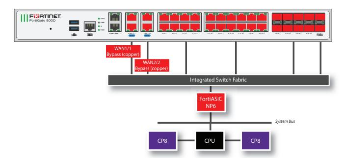
You can use the following get command to display the FortiGate 800D NP6 configuration. The command output shows one NP6 named NP6\_0. The output also shows all of the FortiGate 800D interfaces (ports) connected to NP6\_0. You can also use the diagnose npu np6 port-list command to display this information.
