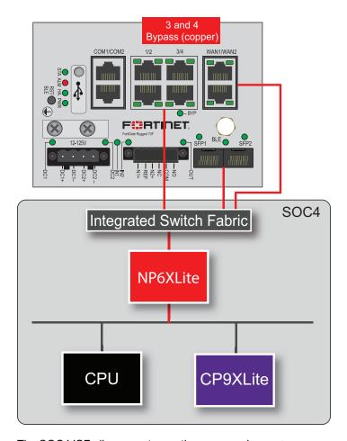
The SOC4 ISF allows you to use the command config system virtual-switch to create a virtual hardware switch that can include any front panel interface connected to the SOC4.
