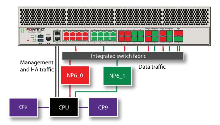
The MGMT interface is not connected to the NP6 processors. Management traffic passes to the CPU over a dedicated management path that is separate from the data path. You can also dedicate separate CPU resources for management traffic to further isolate management processing from data processing (see Improving GUI and CLI responsiveness (dedicated management CPU) on page 23).
