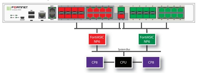
You can use the following get command to display the FortiGate 900D NP6 configuration. The command output shows two NP6s named NP6\_0 and NP6\_1. The output also shows the interfaces (ports) connected to each NP6. You can also use the diagnose <code>npu np6 port-list</code> command to display this information.
