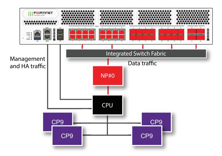
The MGMT interfaces are not connected to the NP7 processor. Management traffic passes to the CPU over a dedicated management path that is separate from the data path. You can also dedicate separate CPU resources for management traffic to further isolate management processing from data processing (see Improving GUI and CLI responsiveness (dedicated management CPU) on page 23).
