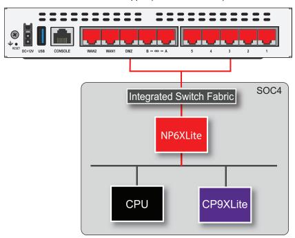
The SOC4 ISF allows you to use the command <code>config system virtual-switch</code> to create a virtual hardware switch that can include any front panel interface connected to the SOC4.
