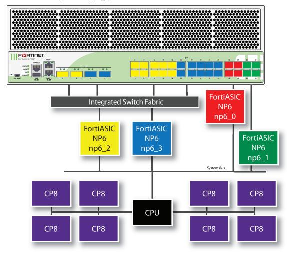
You can use the following get command to display the FortiGate 3700D NP6 configuration. In this output example, the first two NP6s (np6\_0 and np6\_1) are configured for low latency. The command output shows four NP6s named NP6\_0, NP6\_1, NP6\_2, and NP6\_3 and the interfaces (ports) connected to each NP6. You can also use the <code>diagnose npu np6 port-list</code> command to display this information.
