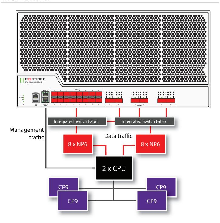
The FortiGate 3960E includes sixteen NP6 processors (NP6\_0 to NP6\_15). All front panel data interfaces and all of the NP6 processors connect to the integrated switch fabric (ISF). All data traffic passes from the data interfaces through the ISF to the NP6 processors.
