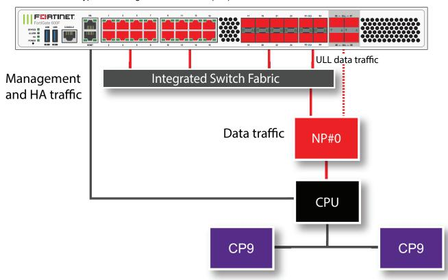
The MGMT interface is not connected to the NP7 processor. Management traffic passes to the CPU over a dedicated management path that is separate from the data path. You can also dedicate separate CPU resources for management traffic to further isolate management processing from data processing (see Improving GUI and CLI responsiveness (dedicated management CPU) on page 23).
