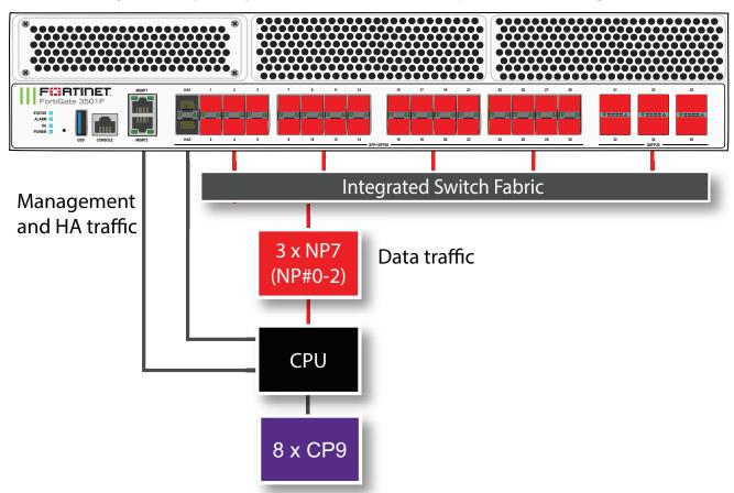
The MGMT interfaces are not connected to the NP7 processors. Management traffic passes to the CPU over a dedicated management path that is separate from the data path. You can also dedicate separate CPU resources for management traffic to further isolate management processing from data processing (see Improving GUI and CLI responsiveness (dedicated management CPU) on page 23).
