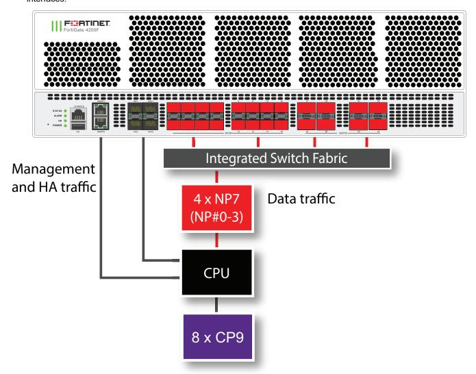
The MGMT interfaces are not connected to the NP7 processors. Management traffic passes to the CPU over a dedicated management path that is separate from the data path. You can also dedicate separate CPU resources for management traffic to further isolate management processing from data processing (see Improving GUI and CLI responsiveness (dedicated management CPU) on page 23).
