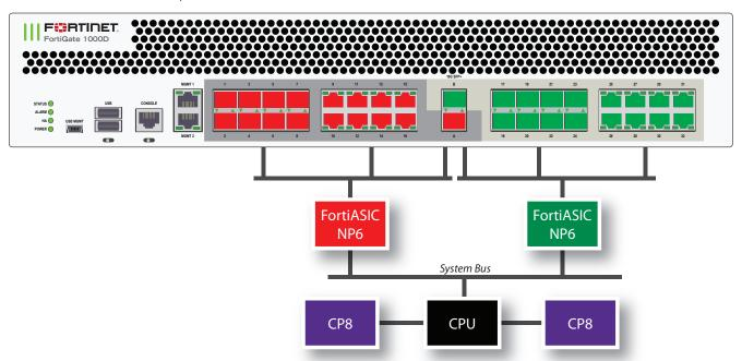
You can use the following get command to display the FortiGate 1000D NP6 configuration. The command output shows two NP6s named NP6\_0 and NP6\_1. The output also shows the interfaces (ports) connected to each NP6. You can also use the diagnose npu np6 port-list command to display this information.
