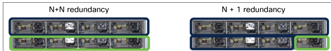
Figure 10. Power redundancy modes
