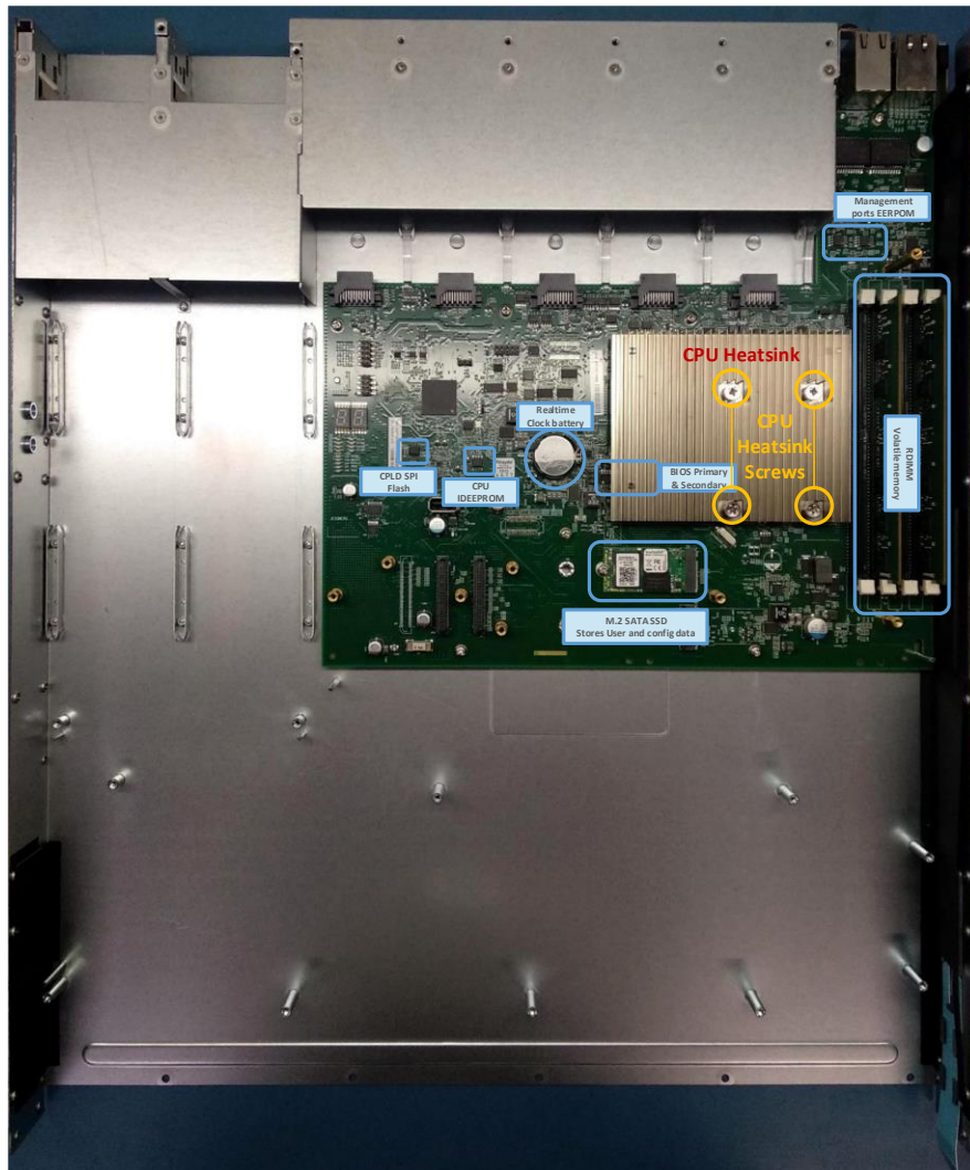
Figure 13 CPU Board volatile and non-volatile memory devices
