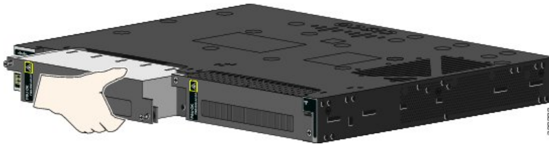
Figure 27: Removing the Power-Supply Blank
