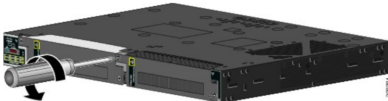
Figure 34: Removing the Screws
