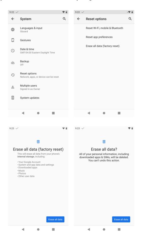
If the Cisco Wireless Phone 840 or 860 is not able to boot properly, a factory reset can also be initiated via the following procedure:
