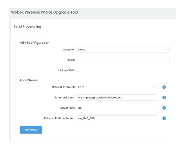
To connect to a PSK enabled Wi-Fi network, enter the **SSID**, set **Security** to **WPA2-Personal**, then enter the 8-63 ASCII or 64 HEX **Password**.
