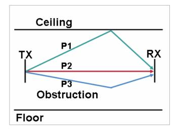
Use of Orthogonal Frequency Division Multiplexing (OFDM), which is used by 802.11a/n/ac and 802.11g/n, can help to reduce issues seen in high multipath environments.
