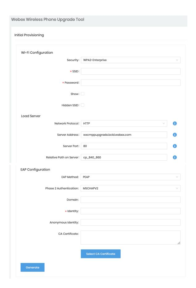
**Note:** A non-broadcasted Wi-Fi network must be configured as a **Hidden SSID**; otherwise the Wi-Fi network will show as not in range. Set **Hidden SSID** to **True** to connect to a non-broadcasted Wi-Fi network.
