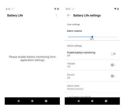
To enable battery life monitoring, ensure the slider for **Enable battery monitoring** is to the right to be set as **On**. The number of full charge cycles can also be viewed.
