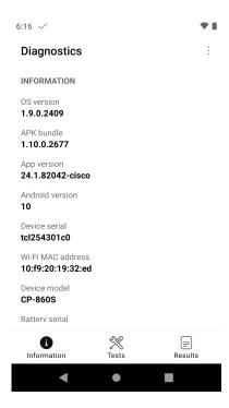
To run select hardware troubleshooting, select the Tests tab, then select the desired hardware component.
