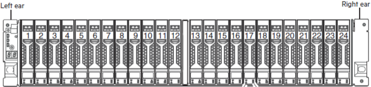
Figure 1: 24-drive enclosure or expansion enclosure—front panel with hubcaps removed
