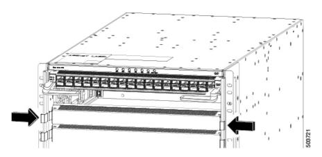
b) Hold the blank line card using both the hands and pull the blank line card completely out of the chassis slot.
