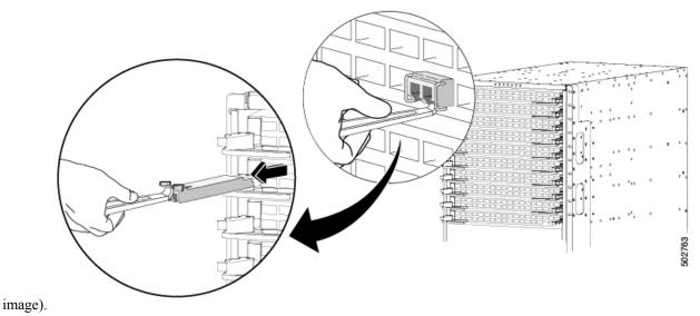
**Step 4** Place the transceiver module in an antistatic bag or other protective environment.
