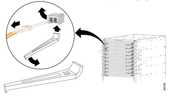
Step 3 Use the narrow end of the optics extraction tool to carefully remove the transceiver module (see the following
