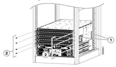
Handles used to adjust the chassis 2 placement.
