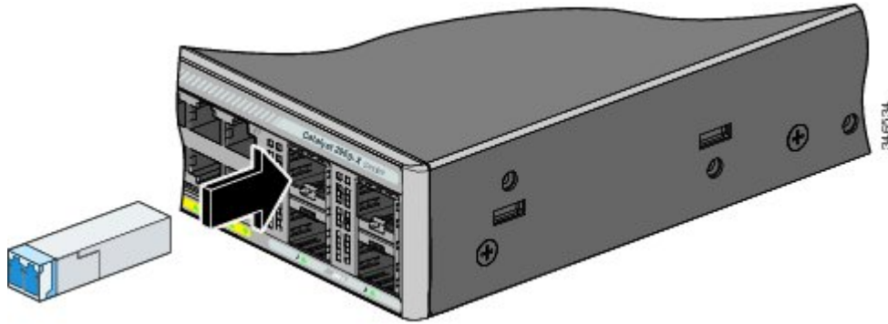
Figure 23: Installing an SFP Module
