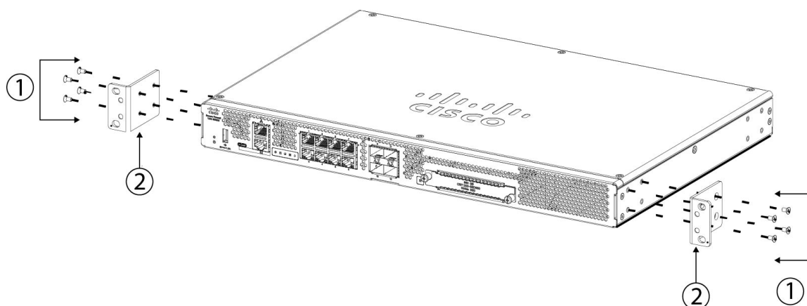
Figure 28: Attach the Rack-Mount Brackets to the Chassis
