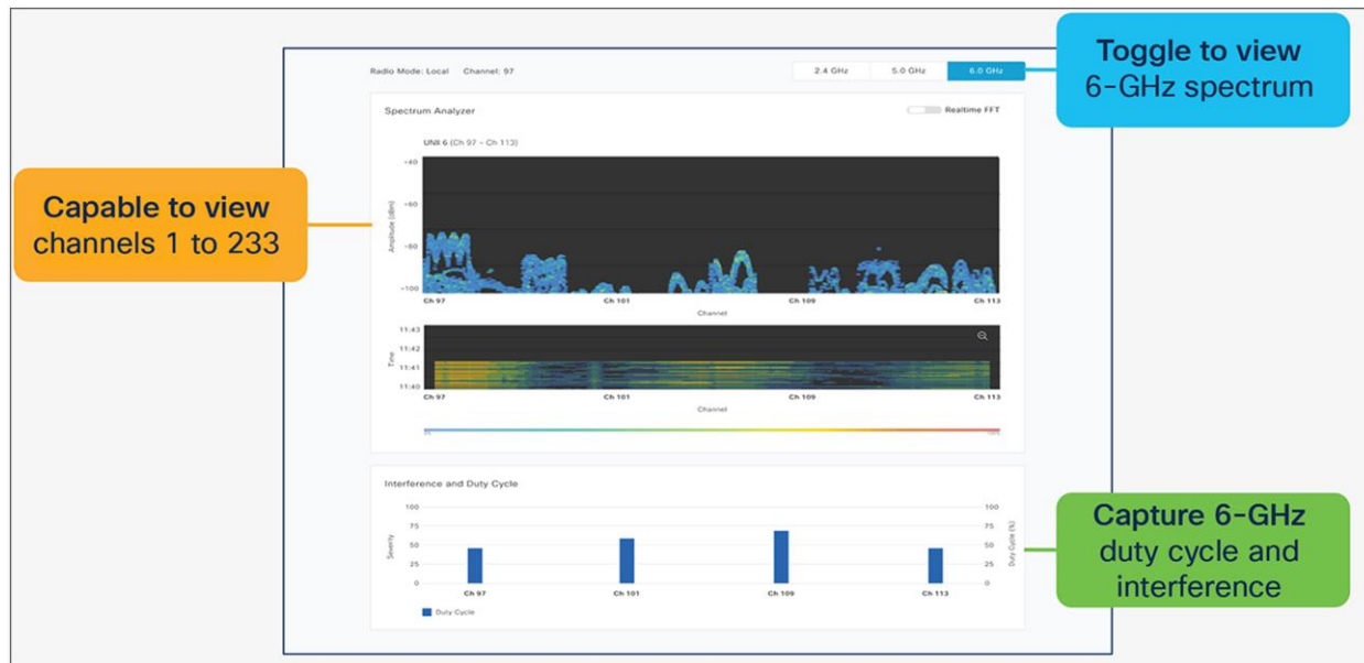
Figure 61. Spectrum analysis: Visualize RF spectrum energy, not only for 2.4-, 5-, and 6-GHz bands
