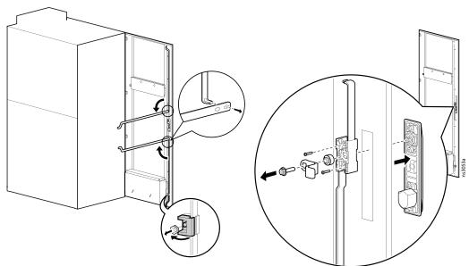
The gear box can be installed on a rack door to accommodate a NetBotz Rack Access handle kit
