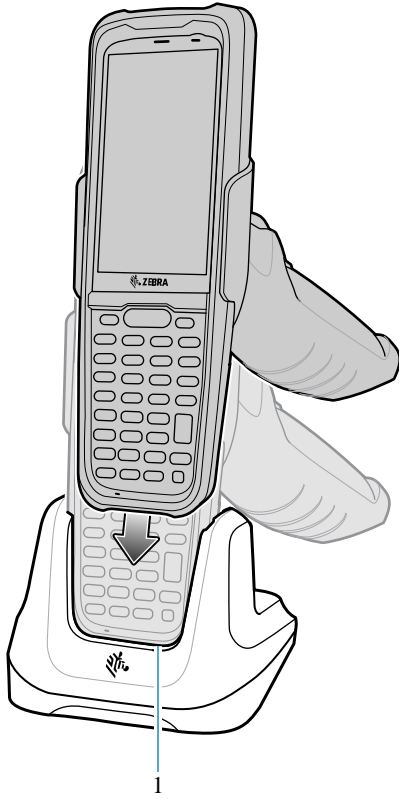
Figure 21 1-Slot Charge/USB Cradle
