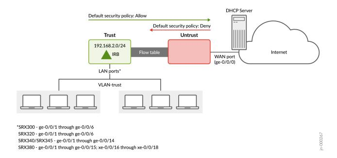
While the port type and count varies between branch SRX models (SRX 300 Series), the factory default configuration results in the same type of connectivity:
