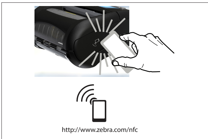
Figure 27 • Near Field Communication (NFC) Pairing
