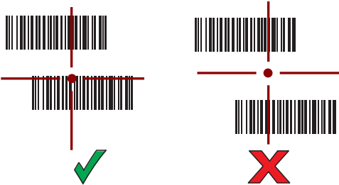
Figure 13 RS507/RS507X Pick List Mode with Multiple Barcodes in Aiming Pattern
