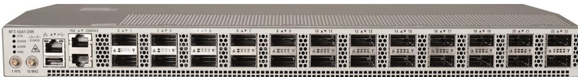
Figure 2. The Cisco NCS-55A1-24H Chassis
