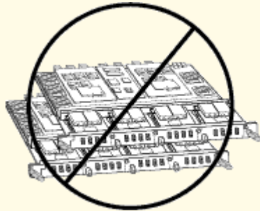
Figure 252: Do Not Stack FPCs
