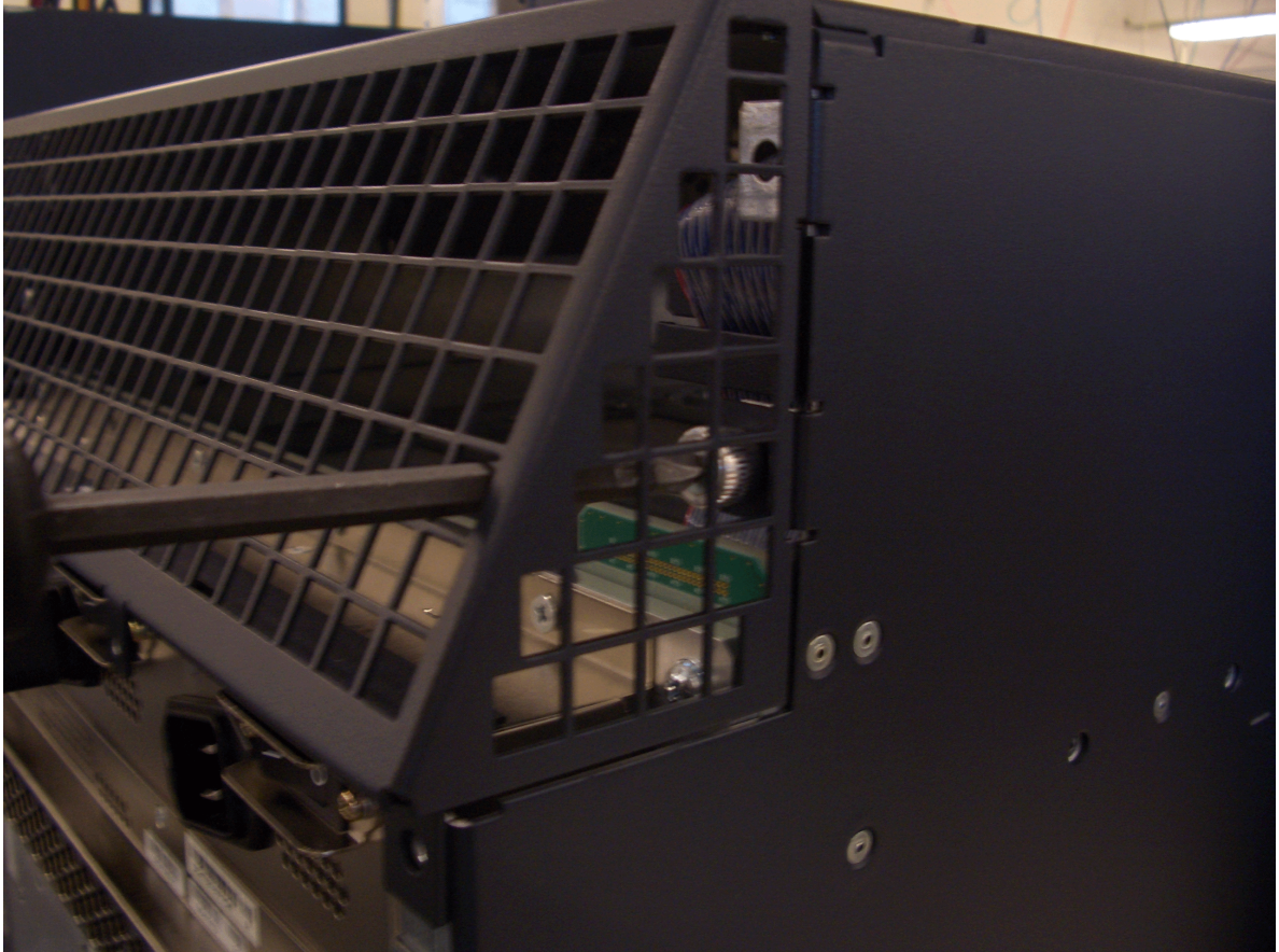
Figure 84: Removing the Right Captive Screw of the Rear Air Exhaust Grate
